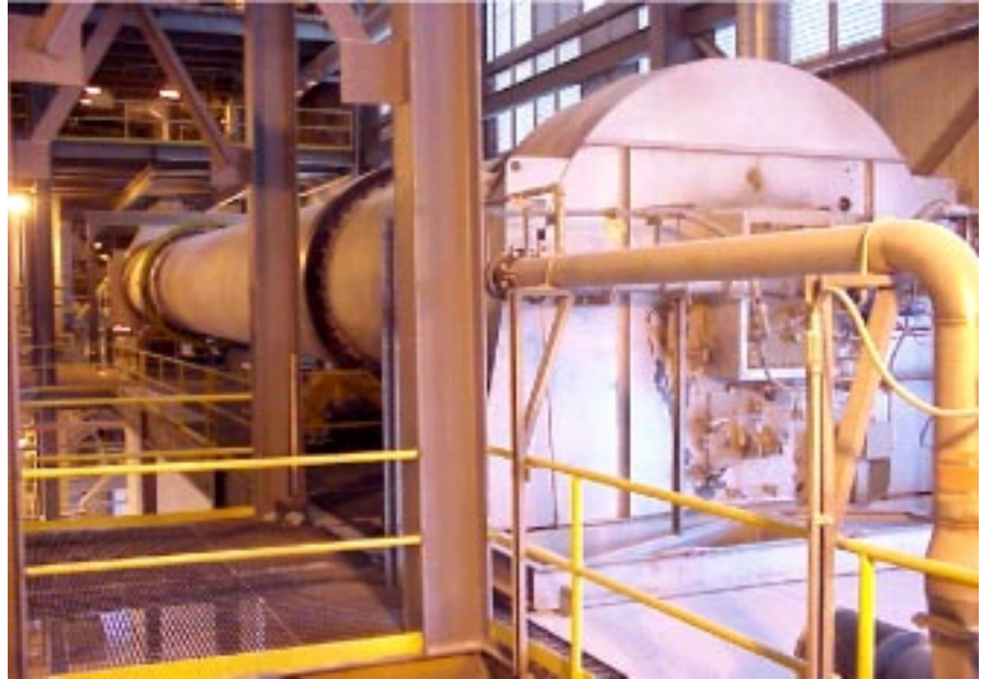
102" diameter x 100' long Bartlett-Snow™ Rotary Kiln
