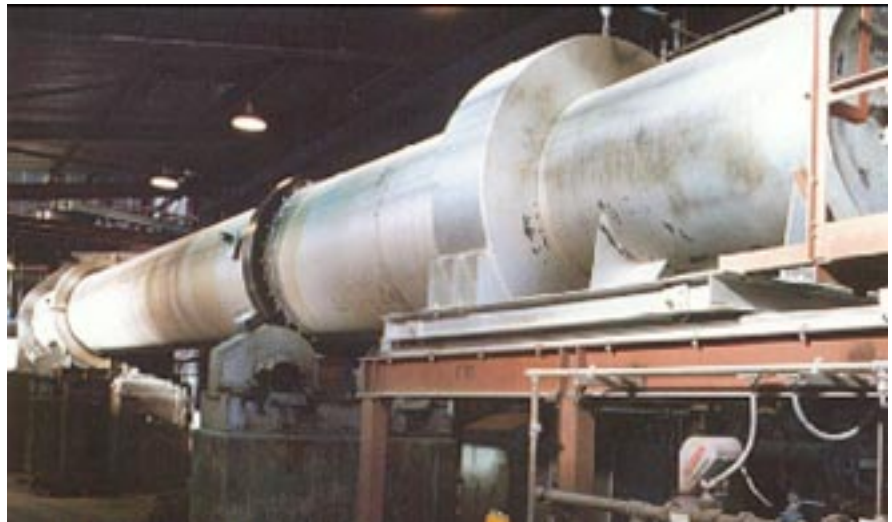
60" diameter x 65' long Bartlett-Snow™ Rotary Kiln
